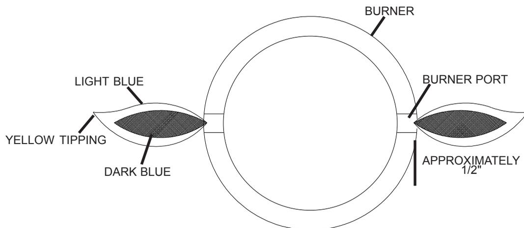
If the burner is getting too little air, the flames will be lazy yellow, and possibly produce soot. If the burner is getting too much air, the flames will be lifting erratically from the burner and may cause difficulties when lighting.
